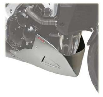
FIX THE ABS ENGINE SPOILER WITH ITS SCREWS KIT 4X10, WASHERS AND NUTS. APPROACH THE ENGINE SPOILER TO THE MOTORBIKE TO FIND THE FIXING POINT; MOUNT THE SPECIF-IC BRACKETS USING THE ORIGINAL SCREWS OF CARTER WITHOUT LOCKING (SEE THE PICTURES); MOUNT THE ENGINE SPOILER ON THE BRACKETS USING THE 5X16 SCREWS AND THE RUBBER WASHERS BETWEEN THE ENGINE SPOILER AND THE BRACKET.
